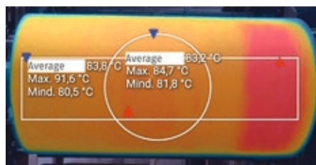
Fig. 18: Thermographs of an operating test for profiling at 100 % power. The machine only accelerated by 3.5 %, not the expected 10 % to 14 %. The leading edge is almost 9°C warmer 22
