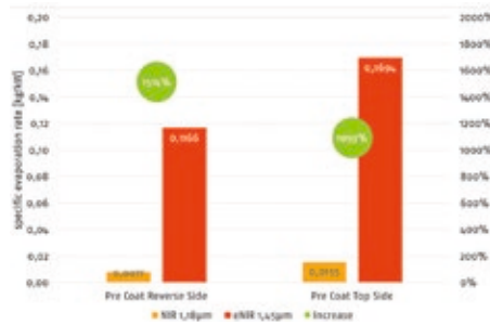
Fig. 12: Change in the specific evaporation rate as a function of the capillarity of the substrate depending on the wavelength of the emitter 18
