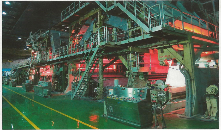
Fig. 2: Compact Engineering’s IRE at the 1st and 2nd coater head in the foreground, Impact’s emitter on the top coating in the background
